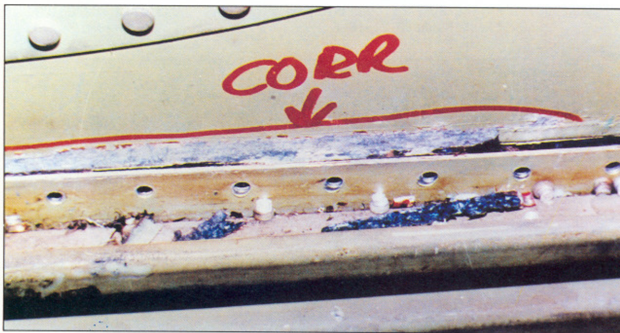
FIGURE 5-10. REMOVAL OF FILLET SEAL FROM INTERNAL EDGE OF LAP JOINT EXPOSED FULL EXTENT OF CORROSION
