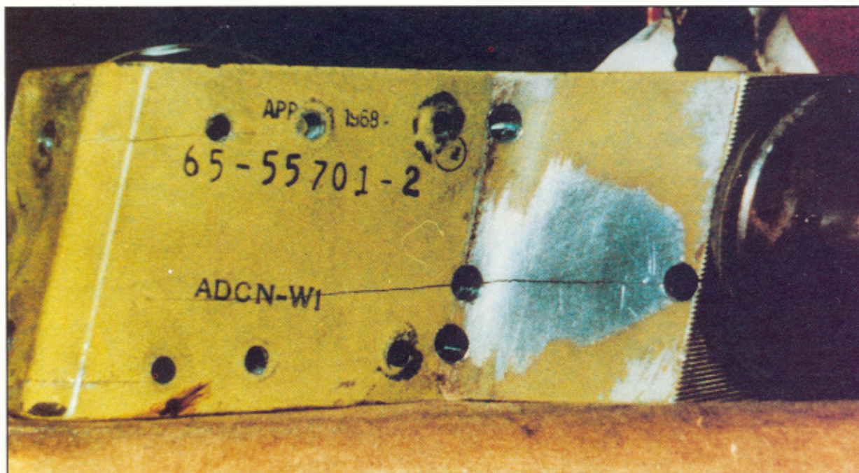
FIGURE 2-12. STRESS-CORROSION CRACKING OF 7079-T6 FITTING
