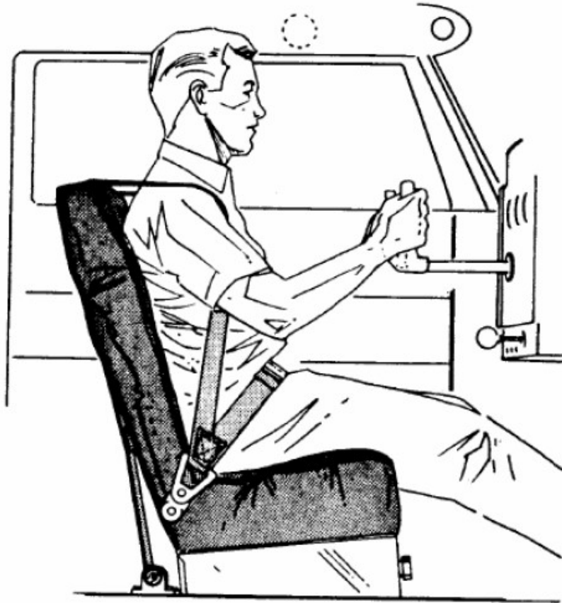
Figure 10-11. Floor Mounted Inertia Reel—Double Over-the-Shoulder Type Harness
