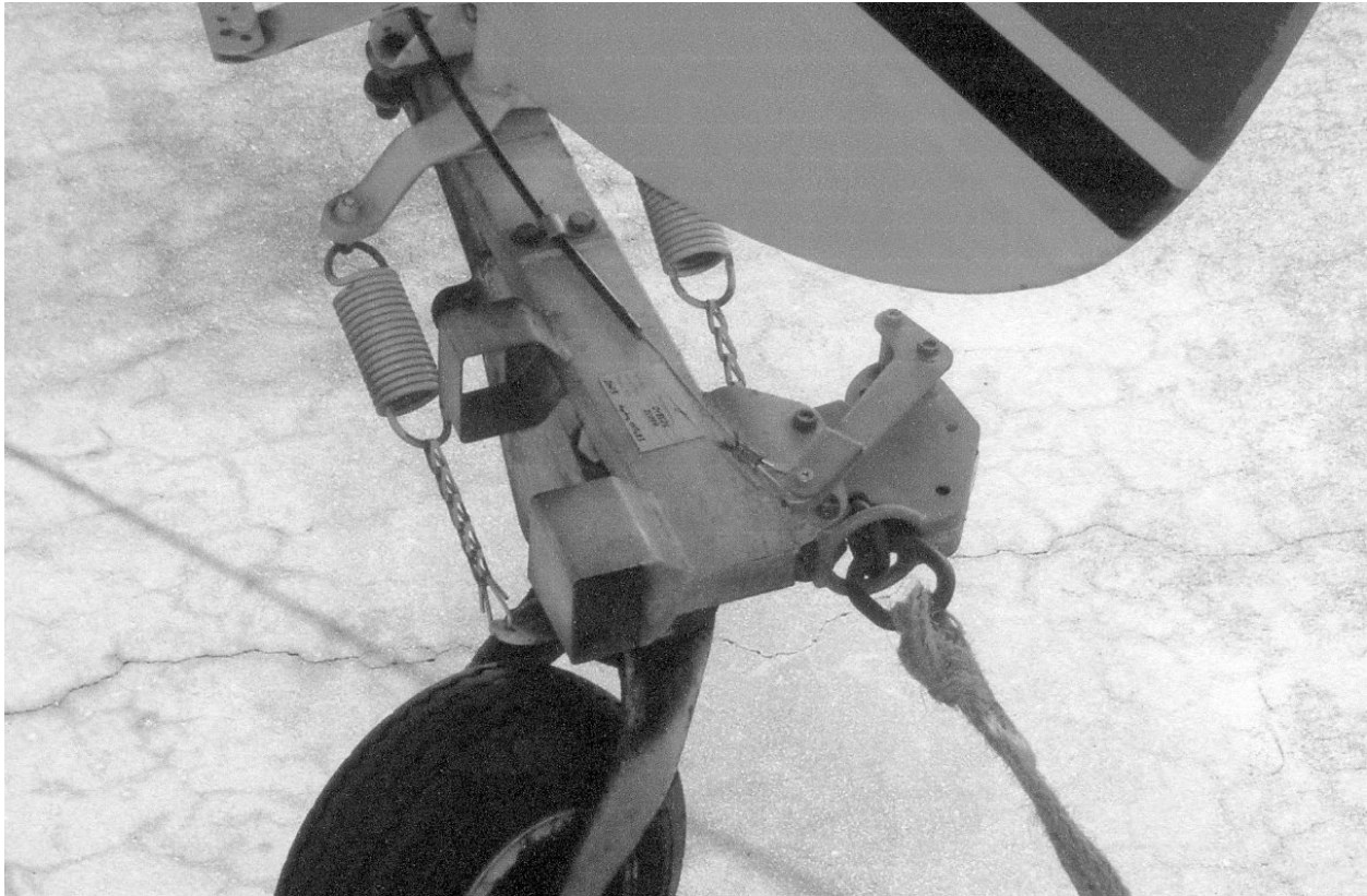
Figure 9-13. Typical TOST Conventional Leaf Spring Mount
