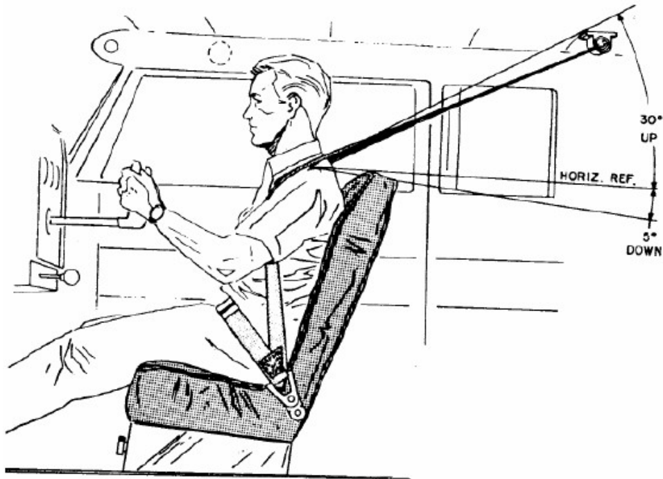
Figure 10-7. Ceiling Mounted Inertia Reel—Double Over-the-Shoulder Type Harness
